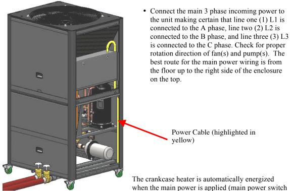
in the ON (|) position. It should be on for at least 24 hours before startup to force dissolved refrigerant from the compressor oil.
